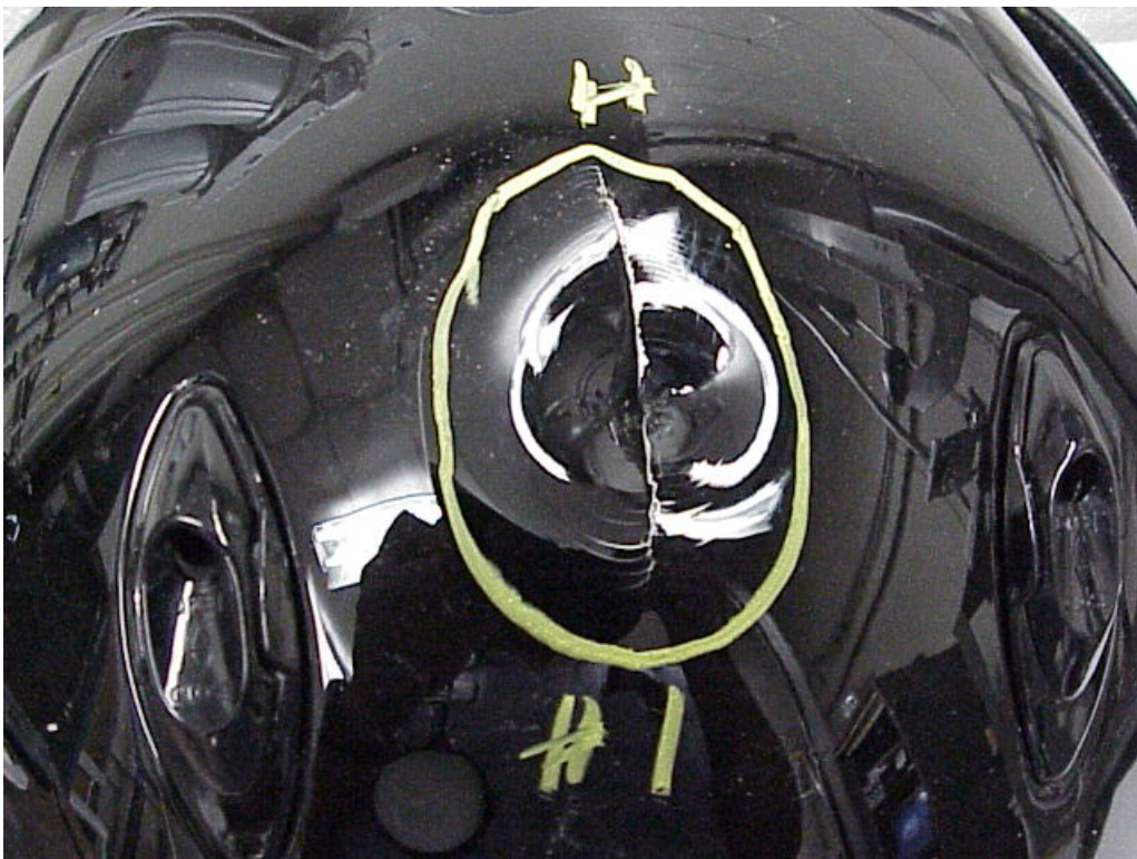
Helmet Photograph 16 Penetration Failure – High Temperature AFX, FX-28, S (56-57 cm)
