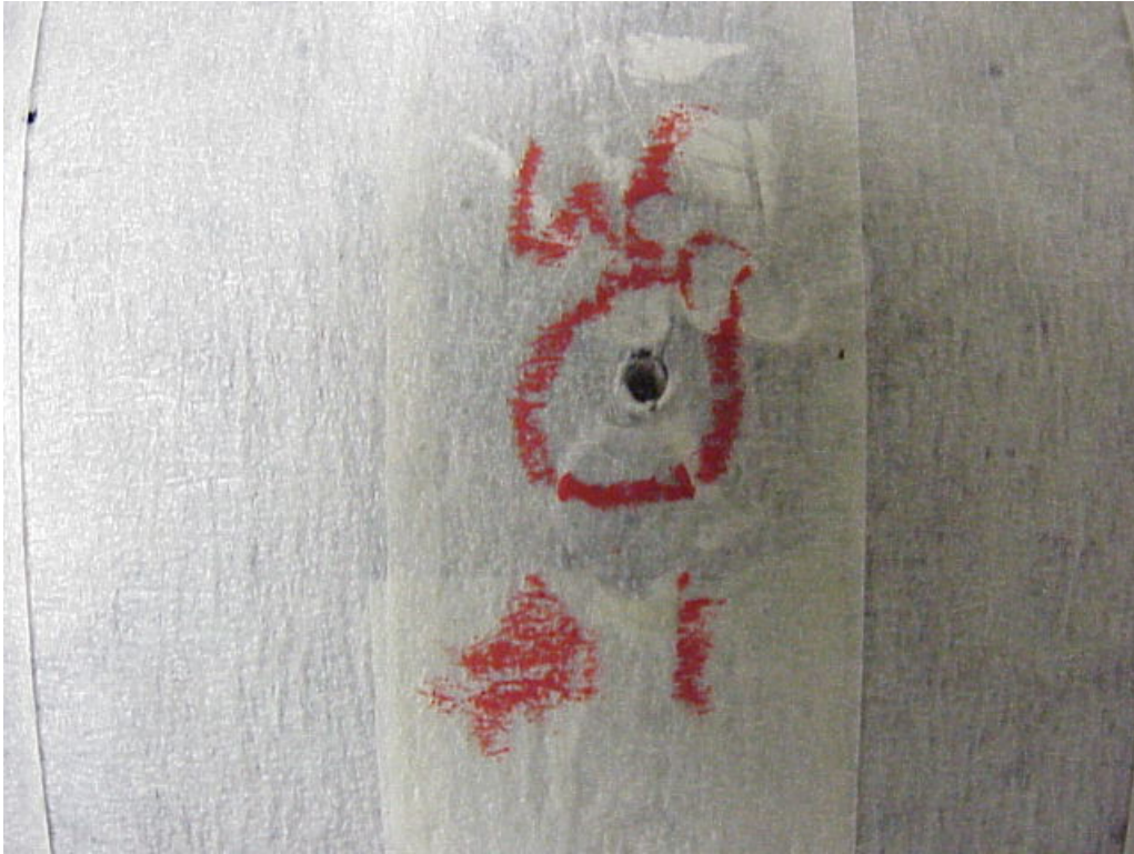
Helmet Photograph 17. Penetration Failure – Water Immersed AFX, FX-28, S (56-57 cm)
