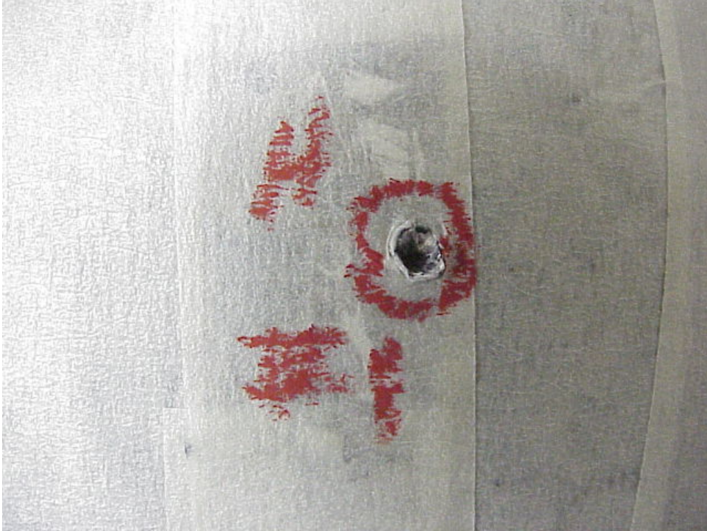
Helmet Photograph 15. Penetration Failure – High Temperature AFX, FX-28, S (56-57 cm)
