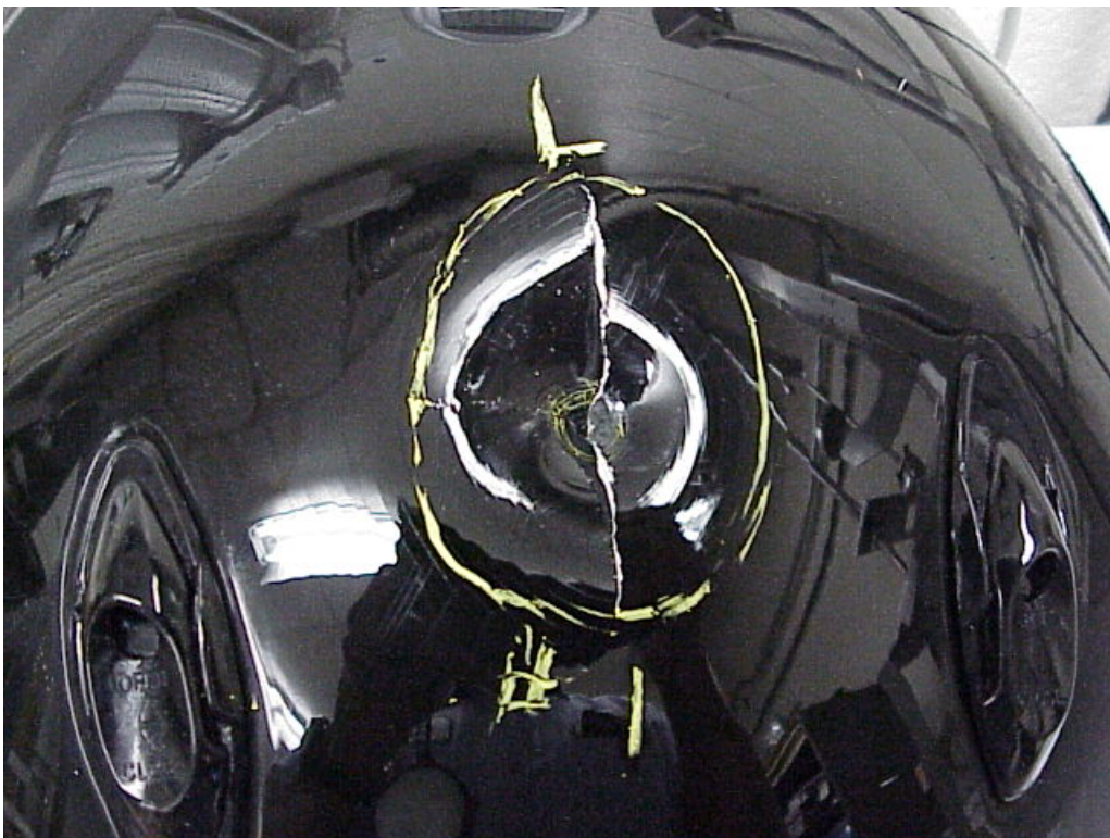
Helmet Photograph 14. Penetration Failure – Low Temperature AFX, FX-28, S (56-57 cm)
