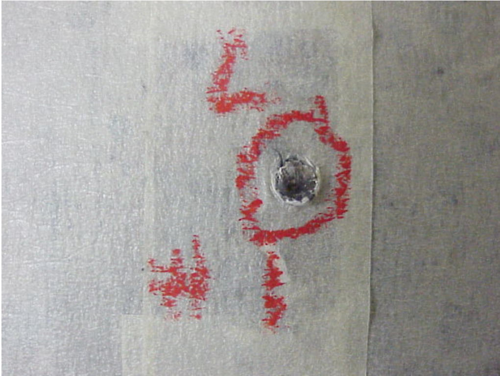
Helmet Photograph 13. Penetration Failure – Low Temperature AFX, FX-28, S (56-57 cm)
