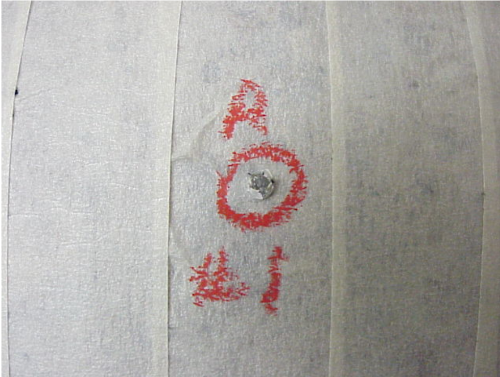
Helmet Photograph 11. Penetration Failure - Ambient AFX, FX-28, S (56-57 cm)
