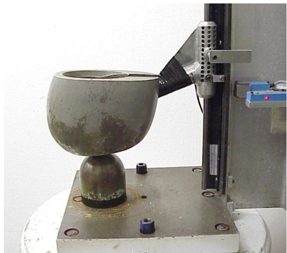
SwRI Helmet Test Equipment Photo 3. Hemispherical Anvil Impact Configuration
