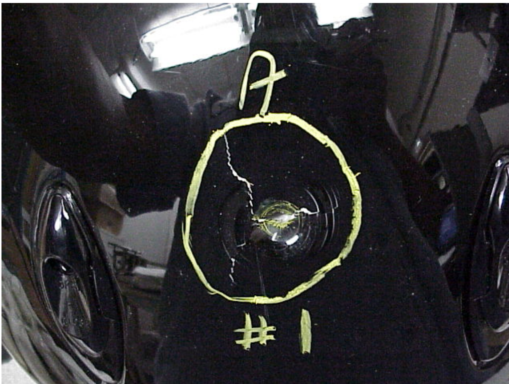
Helmet Photograph 12. Penetration Failure - Ambient AFX, FX-28, S (56-57 cm)
